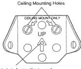
The nail hole is for positioning only.
